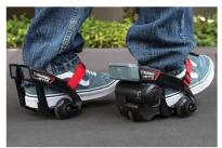
When strapped on, the rear wheel of the powered skates are designed to be positioned slightly above the ground, so you can still walk normally even with the darn things on. To start skating, simply put your
